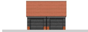
TWIN GARAGE FRONT ELEVATION 1 : 100
